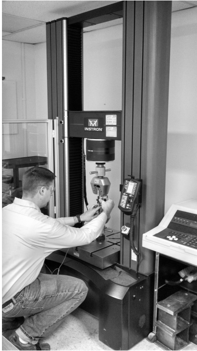
Coupon testing is conducted to verify mechanical properties.
