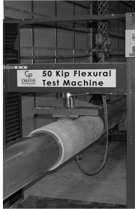
Full section bending test is conducted to assure product performance.
